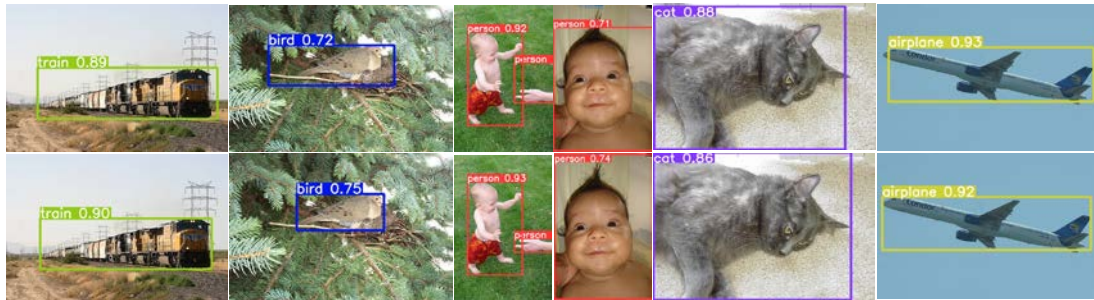
Fig. 8. Quality comparison of bounding box predictions. The objects with detection scores higher than 0.5 are shown. In each pair, the top is the detection results of CenterNet, and the bottom is our improved model.
